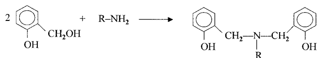
Figure 7 Formation of dibenzylamine bridges between phenolic groups as a result of reaction of methylol groups with amines. 6
